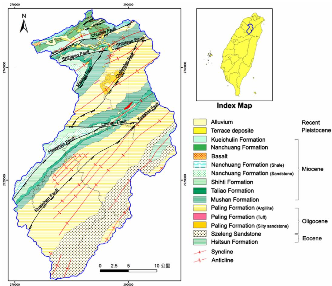
Fig. 1 Geological map of the Shihmen Reservoir catchment area
